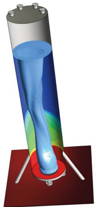
Multiphase mass fractions in a three-phase bubble column as analyzed with ANSYS FLUENT software
